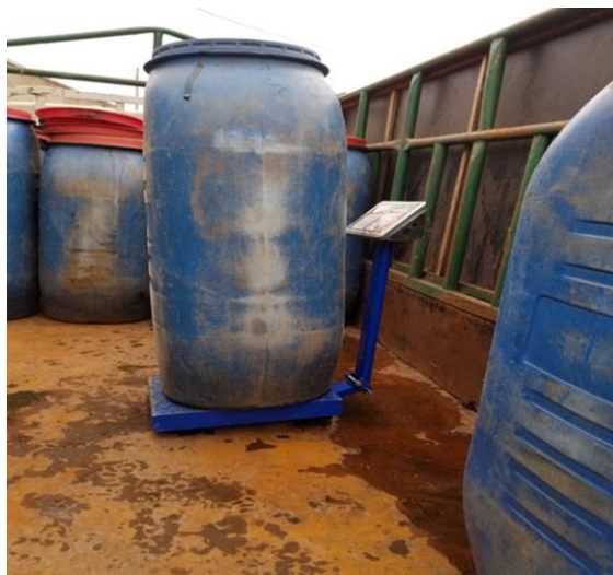
Figure 3-5: a drum containing sludge being weighed on an automatic scale
