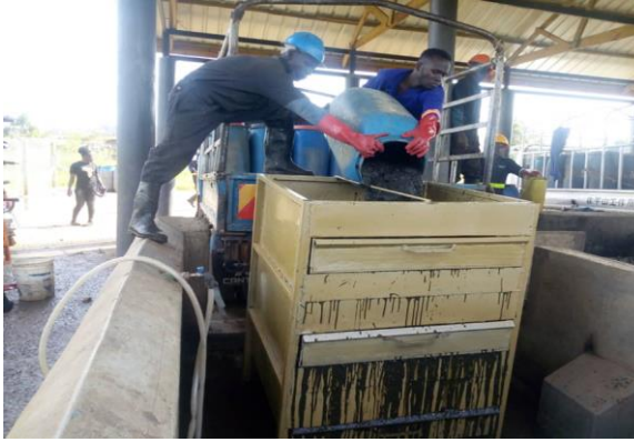
Figure 3-6: drum containing sludge is emptied into the sieve
